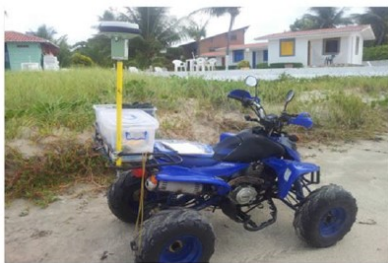
Figure 1. Kinematic Survey equipment (Receiver connected to the quadricycle)
